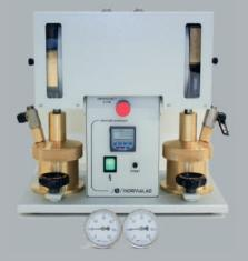
For the preparation of grease sample, the GWM Classic assist to work the grease used for the preparation of shear stability test. It is a compact twin-unit automatic grease worker using electronic counter to control the strokes number. The GWM Classic is suitable for single or double worker operation.
