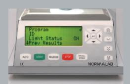
Thanks to an integrated software, you can easily program the parameters through an access keypad. The parameters characterizing a test are gathered in tables. Up to 20 tables can be memorized by the user according to the preferences and the samples. Parameters to set:
